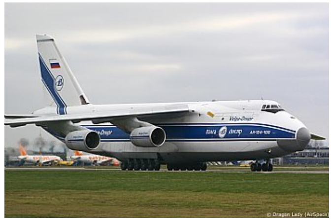
The Antonov 124 is one of the largest cargo planes, with a cargo compartment of 36 m x 6.4 m x 4.4 m
