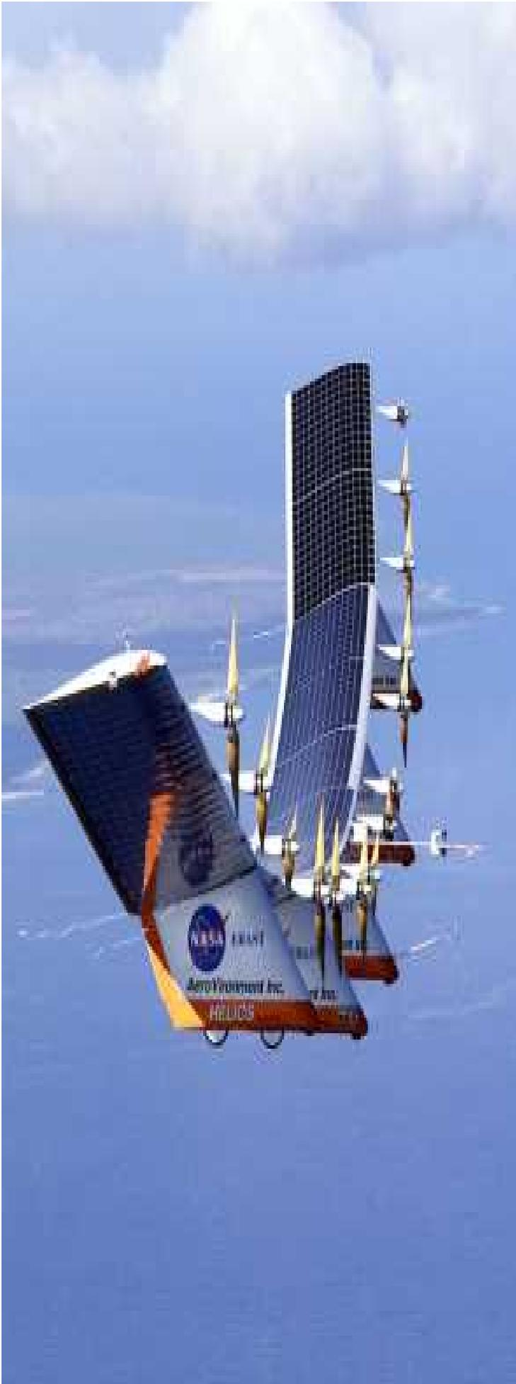
An unmanned solar-powered aircraft set a world altitude record of 96,500 ft. in August 2001.
